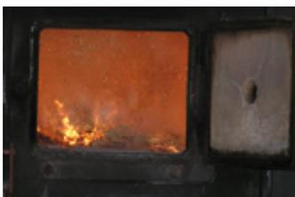
The "bagasse" produces all of the energy (heat) necessary for the production of rum and runs the steam turbines that operate the mill, by transforming the steam (300 - 350° C (572 - 662° F) into electricity. The mills operate in the morning, and when they close at the end of the day, they store the "bagasse" for the next day.
